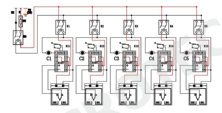
$K_0$ : Power Switch K11-K15: Individual Limit FU:Fuse EH $_1$ EH $_2$ :Heating Pipe K1-K5: Individual Power Switch C1-C5: Buzzer A(B): Thermocouple 618T: Digital Controller
