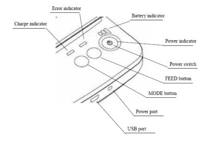
[CHARGE]:Battery charge indicator [ERROR]:Error indicator
